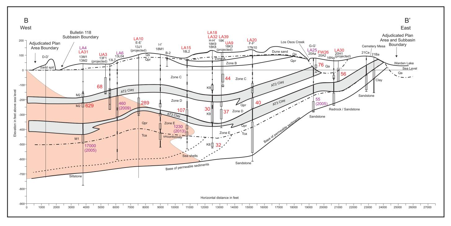
Aquifer Zones: Zone A - Perched Aquifer Zone B - Transitional Aquifer Zone C - Upper Aquifer Zone D - Lower Aquifer (shallow) Zone E - Lower Aquifer (deep) Well data point
