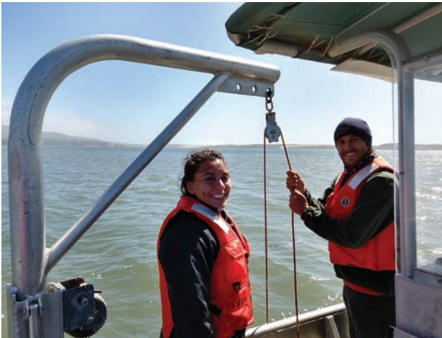
In this picture, Sydney Wewerka (left) and Professor Walter (right), lower a sampler into the bay to gather sediment from the bay bottom. Samples are sent to a lab to conduct grain size analysis.
