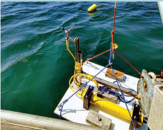
Cal Poly researchers lower an array of water quality sensors into the bay where they will continuously gather data for one month. The measurements include temperature, water velocity, and salinity.
