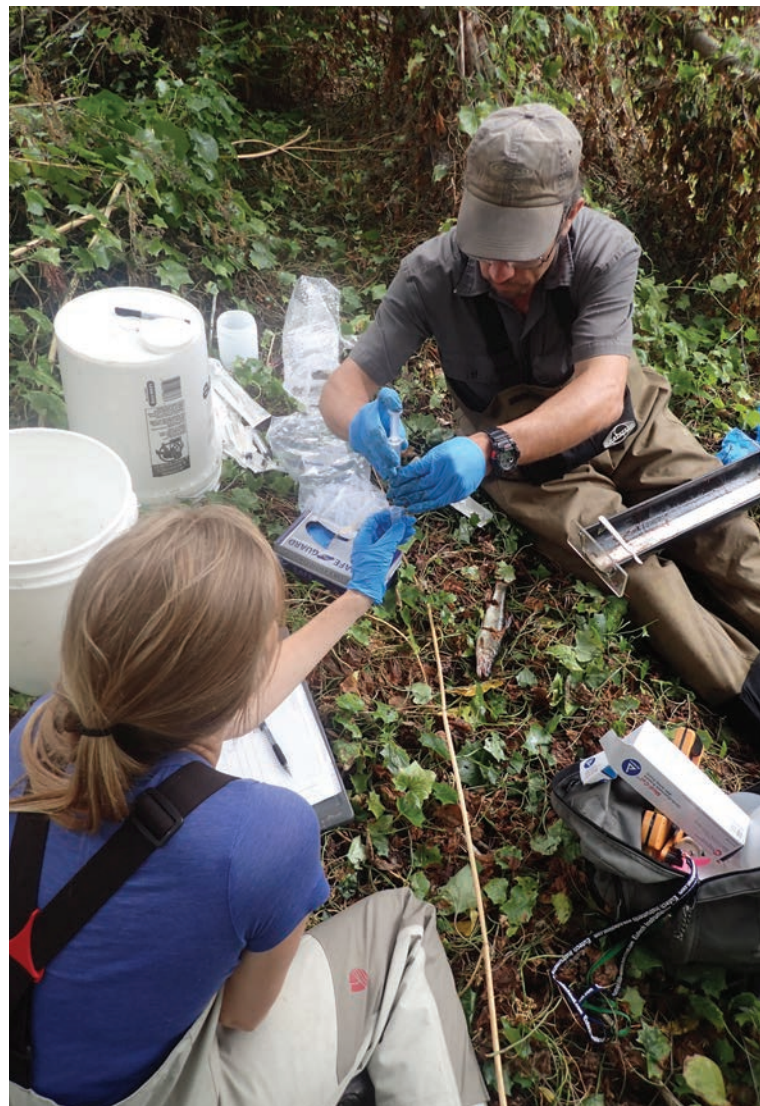
Stillwater Sciences and Estuary Program staff use sterile technique to collect a water sample for eDNA analysis. Photo courtesy of Stillwater Sciences.
