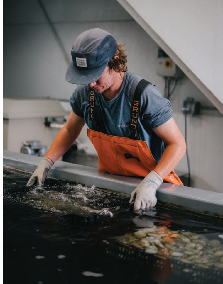
The Morro Bay Oyster Company's depuration facility consists of tanks, pumps, and filters that treat water from the bay to ensure that it is clean. Oysters can be pulled from the bay when waters are not clean enough for harvesting and after filtering in the facility's tanks, the oysters are then clean enough for market. Photo courtesy of Nash Moreno.
