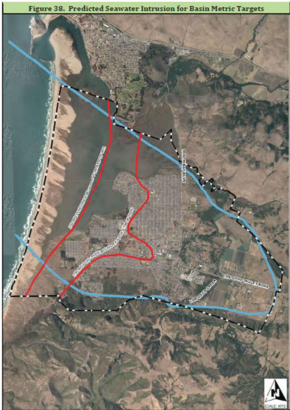
Figure 2. Figure 38 from Basin Plan illustrating seawater intrusion front at BYM 100 and BYM 80
