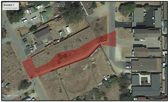
We will locate sufficient monument to plot the location of the right of way lines of Ferrell Avenue and 7<sup>th</sup> Street, along with adjoining property lines that are within the limits of survey. Monuments located as part of the field survey will be shown on the base map.
